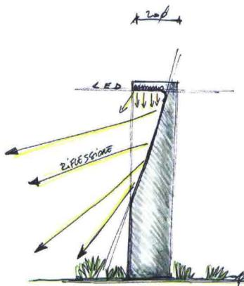
■ An outdoor lamp made of injection-moulded expanded polyurethane, anchored to the floor like a totem. The cylindrical body features a diagonal cut-out section whose white surface reflects and diffuses the light shining down from the 12-Watt LED source. The shade is made of a thermoplastic material. It is 90 cm tall and has a diameter of 20 cm.
